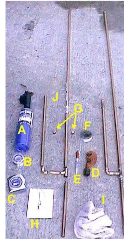
A=Benz-O-Matic propane torch; B=Lead-Free solder; C=Tape measure; D=Tubing cutter; E=Sharpie marking pen; F=Solder Paste; G=caps; H=Hardcopy of the above drawing; I=Wet Towel; J=PreCut, ready to assemble parts of the 2 meter J-Pole.
