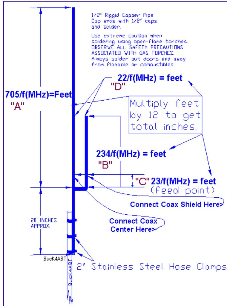
One is for 144 to 148 mHz (model JPOL2) and the other is for 430-450 mHz (model JPOL4). Both models are shown in the following illustration:
