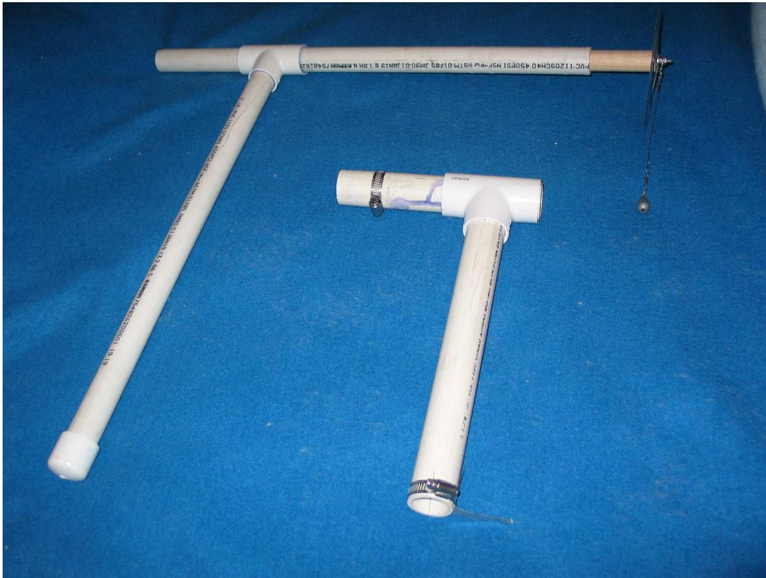
**Boom & Support:** Horizontal Boom and Positioner Arm on Left showing wooden dowel and Elevation Indicator Assembly, Elevation Bearing Assembly on Right (note Hose Clamps for Friction Adjustment)
