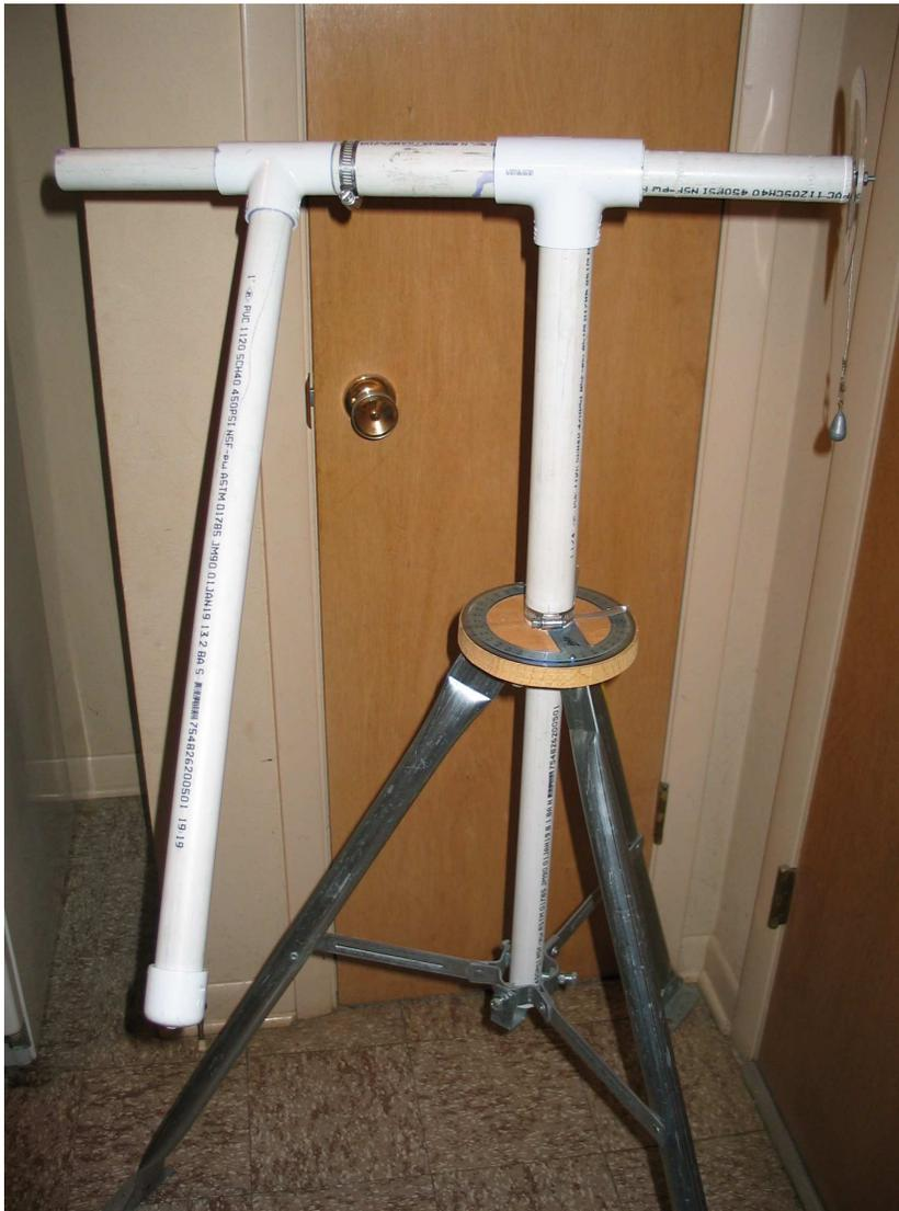
**Complete Positioner:** Complete Positioner Assembly Mounted on Tripod, Dish mounts on Right, Yagi on Left (note Azimuth Pointer)
