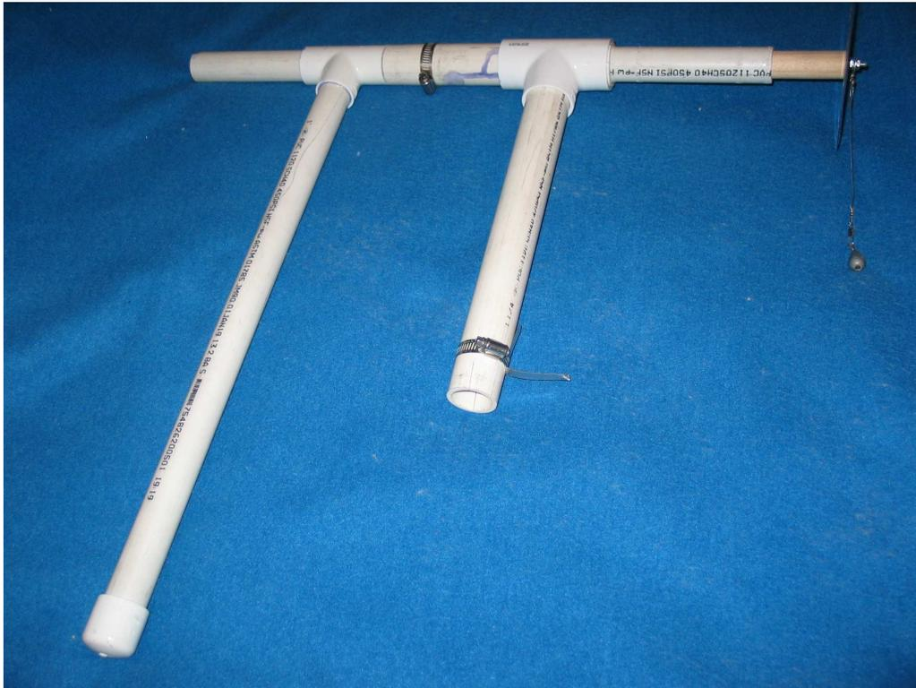
***Positioner: Assembly of Horizontal Boom and Elevation Bearing***
