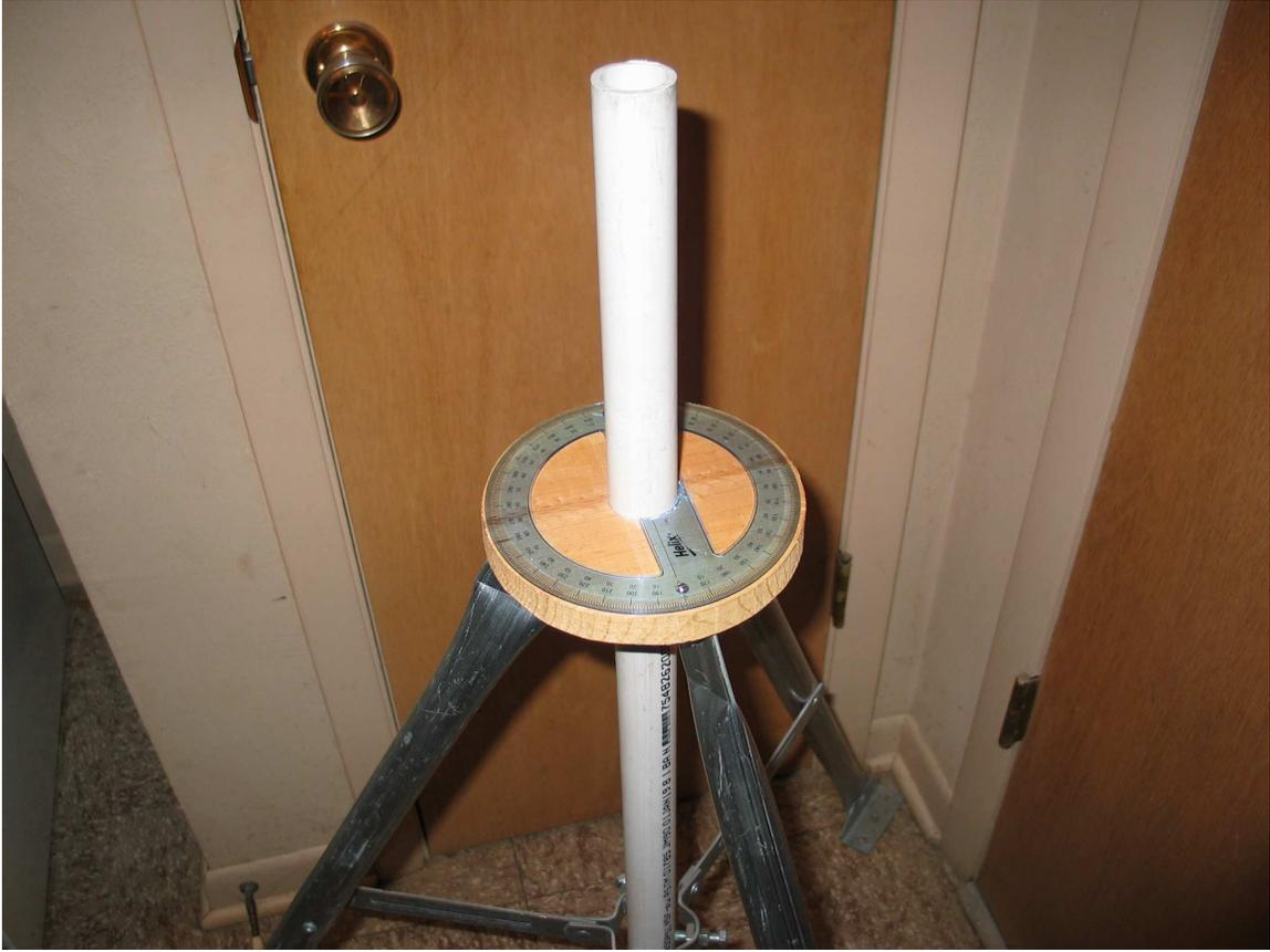
***Tripod: Radio Shack Tripod showing Azimuth Bearing Post and Azimuth Indicator***
